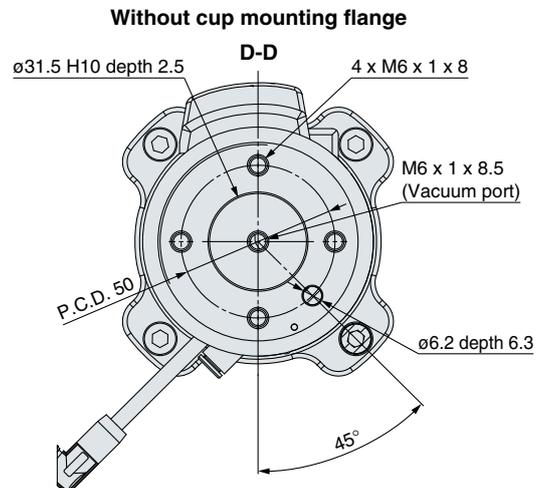
\* The dimensions and mounting method described in this drawing (example) are for the following part number: ZXP7A01-ZPB25JS-X1
