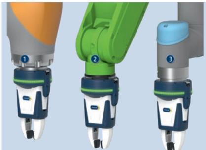
The standard Co-act gripper EGP-C is available for a wide range of collaborative robots (cobots) from a variety of manufacturers including KUKA, Universal Robots and FANUC. The gripper has been pre-configured in a way that it can be mounted directly electrically and mechanically onto the cobots. Depending on the manufacturer, different versions are also available depending on the flange version.
