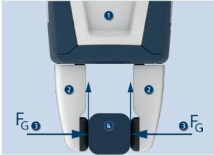
The "gripping force" specification in the catalog refers to the arithmetic sum of the forces acting on each jaw individually at distance P (see illustration). For evaluation of the biomechanical limit values in accordance with ISO/TS 15066, only the gripping force acting on each gripper jaw must be used. Furthermore, the information in the operating manual is referred to.
