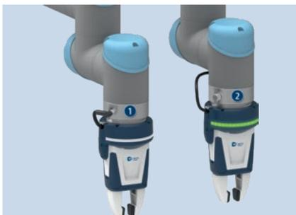
For the robots of the manufacturers Universal Robots and Techman Robot, two variants of the Co-act EGP-C gripper are available. The variants -URID or -TMID use the tool interface of the robot for feed-through of the signals to the robot control system. However, this variant does not have a light band. The light band including the free actuation cannot be used for the variant with external cable routing.
